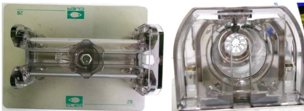
Figure 4-5. A mouse restrainer (CL-4903) tested for the blood collection from tail vein.
