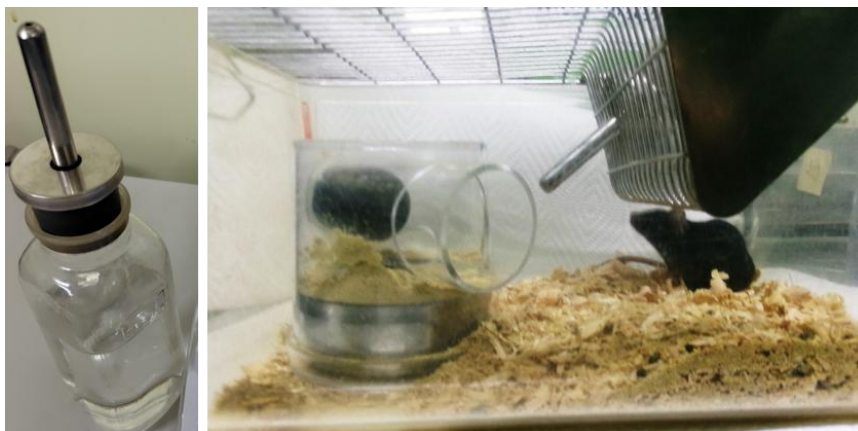
Figure 4-3. Water bottle equipped with a stainless-steel sipper tube (no ball valve type).
